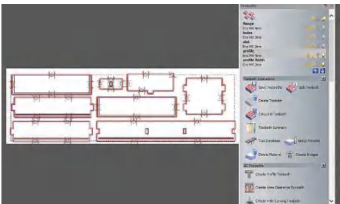
▲ Pic.11 CAM set-up of tool-paths to machine the components
